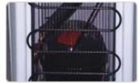
Hermetically sealed reciprocating Compressor
